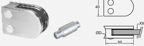
Small D (50 x 40 mm) for Glass 6 to 10.76 mm
