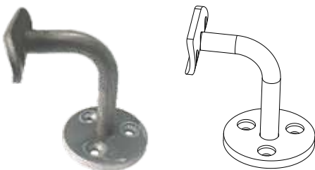
Wall Bracket, Plate 60x6 with 3 holes, Fixed bend Rod 12x75x50 mm, with HRA for Tube 42.4 mm
