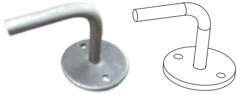
Wall Bracket, Plate 70x6 with 2 holes, 2xØ8.5, Fixed bend Rod 12x75x75mm
