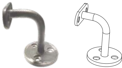
Wall Bracket, Plate 60x6 with 3 holes, Fixed bend Rod 12x75x50 mm, with HRA for Tube Flat
