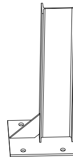
Bolt Down Crash Barrier Post 760 Mm Mild Steel Hot Dip Galvanized
